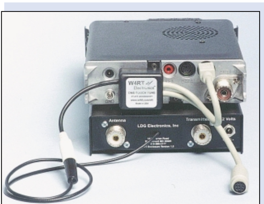
Photo A— Are you weary of having to push a number of buttons just to get a tuning carrier? The newly introduced One-Touch Tune (OTT) is a custom add-on accessory for the Yaesu FT-817 from W4RT Electronics. All you do is press the TUNE button and OTT takes control of the FT-817. (Photo courtesy W4RT Electronics)
