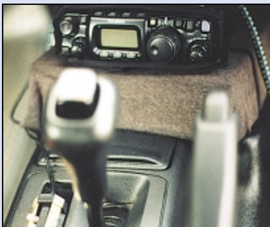
Photo 9— We often take Squeekey mobiling, as it fits perfectly into the gearshift position-display window on my Camaro, and probably many other vehicles. A thin piece of clear double-sided tape on the key's base also holds it solid to a rig case or other surface. Paddle is fitted with cable and 1/8 inch stereo plug for instant use.
