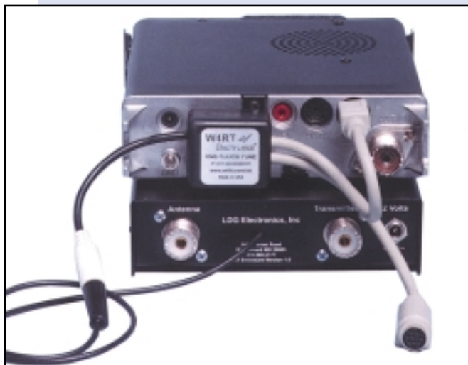
Photo 4—The W4RT Electronics One Touch Tune mod interconnecting a Z11 and FT-817. Mod is ideal for walk-and-talk HF'n where SWR changes as you move. Additional One Touch Tune modules for interfacing LDG's AT-11MP and RT-11 tuners with an FT-897 or TS-50 are also being developed by W4RT Electronics.
