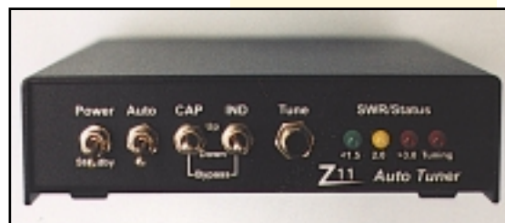
Photo 2— The very popular and widely acclaimed LDG Electronics Z11 Automatic Antenna Tuner. Unit measures 1.5”H × 5”W × 7”D, matches impedances of 6 to 800 ohms, and operates from 13 volts DC or a pair of 9 volt batteries for stand-alone activities. Note SWR-indicating LEDs on front panel. Nice!
