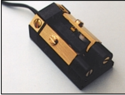
Photo 8— This unique new Squeekey key is handmade by Englmar Wenk, DK1WE, in Germany and is only 1 inch wide by 3 inches long. It sports angled levers, round fingerpieces, and works great with horizontal, vertical, or lateral finger movements. Paddle is rugged with a self-protecting design and is well suited to handheld or off-desk use.
