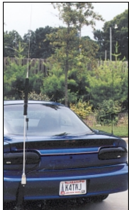
Photo 6— The taller/mobile version of the W6MMA “Super Antenna” is configured with a 22 inch base mast, 14 inch MP-2 motor-driven coil assembly, and 48 inch top whip. Total height is 84 inches. The antenna may be scaled taller or shorter with optional mast and whip sections. (Details in text.)
