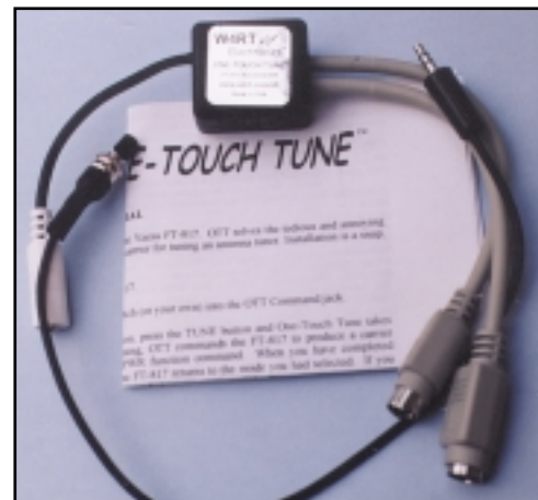
Photo 9— The new “One Touch Tune” module from W4RT Electronics. The unit plugs into sockets on the rear of the FT-817 and a press of its pushbutton or remote activation from an LDG Z11 tuner activate the rig to transmit a tune-up carrier.
