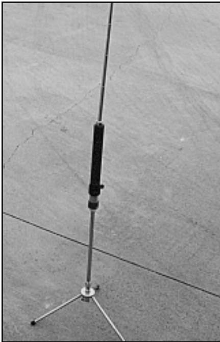
Photo 5— This go-anywhere/portable version of the W6MMA “Super Antenna” consists of a 12 inch base mast, MP-1 manually adjustable coil section, and top whip that extends to 43 inches for operating or retracts to 7.5 inches for carrying. Here the antenna sits on its optional tripod mount. The antenna covers 40 through 2 meters plus 70 cm and also 80/75 meters with an optional coil. It breaks down into 12 inch long sections for traveling.
