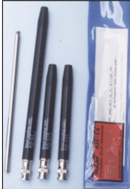
Photo 1—Maldol’s new monoband mini HF antennas utilize a pull-up whip and interchangeable base loading sections to cover 40, 20, 15, and 10 meters. They extend to approximately 50 inches for operating, retract and separate into 7 inch sections for carrying, and are very lightweight. Base sections and extendable whip may be purchased separately to fit your needs.
