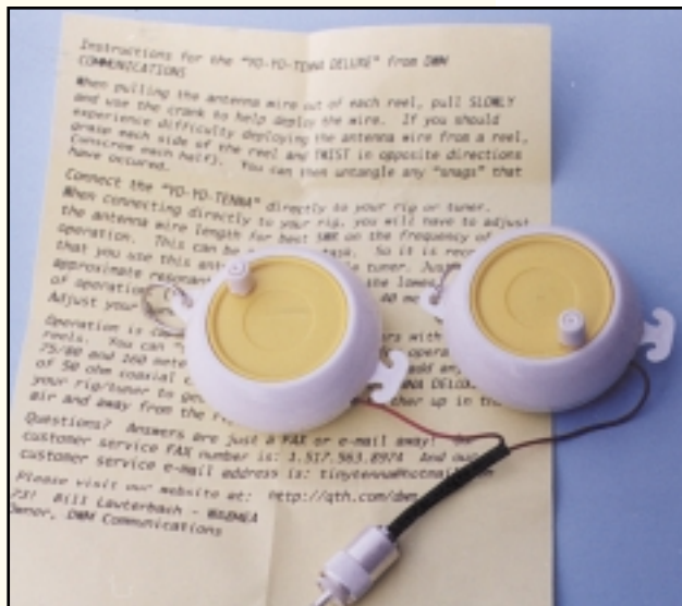
Photo 3— Check out this unique YoYo Deluxe portable antenna from DWM Communications. Each YoYo—err . . . reel—is loaded with 40 feet of insulated wire you pull out to a desired dipole length, then rewind into the reel after use. Wires from each reel connect to the center-located PL-259 you plug into your rig. Clever!
